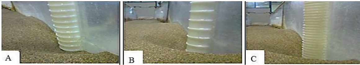
8: Pictures of modeled abutments containing roughness and the hole created around them
