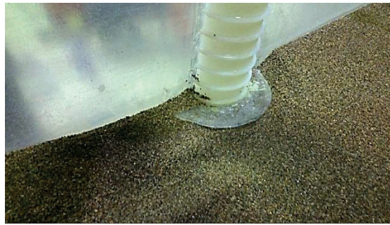
13: The hole created around the abutment containing roughness and collar
