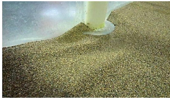
11: Picture of using the collar in abutment and created hole in the experiment
