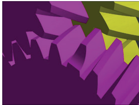
5: Virtual tooth breakage on the pinion of 3 rd speed gear
