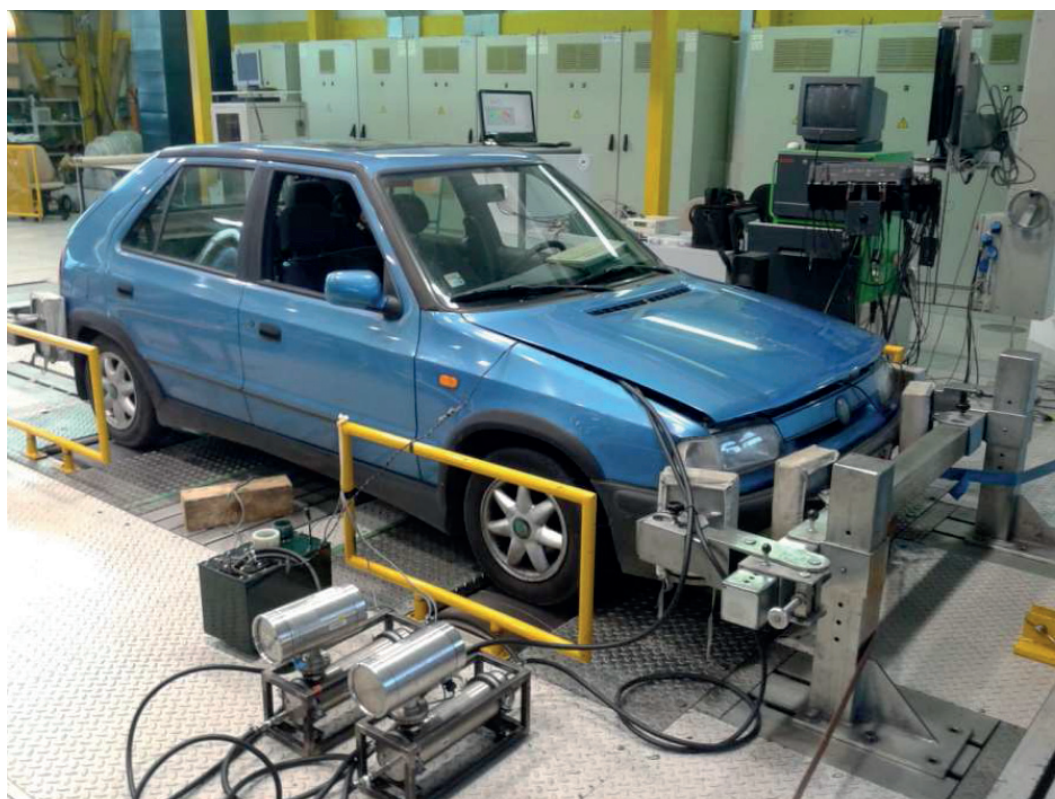
1: Tested Škoda Felicia vehicle on chassis dynamometer
