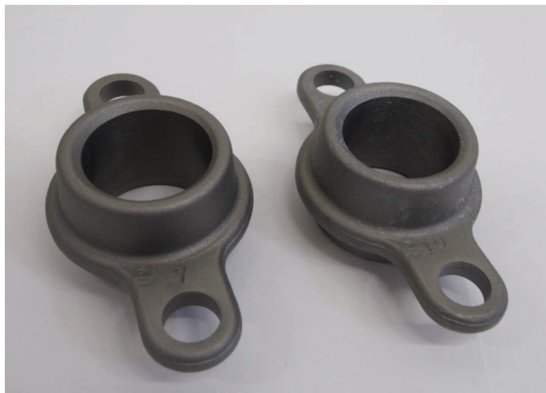
3: The optical result of the first cyclic salt spray test
