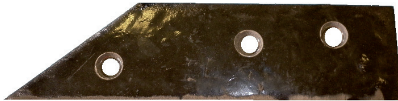
9: Prototype with renovated surface from composite with particles from machining process
