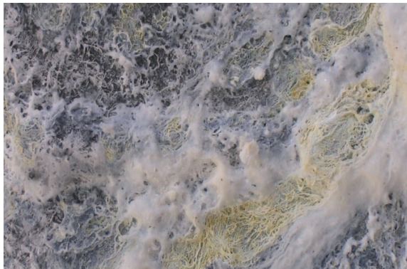
8A: Weld bead protected by hot dipped zinc
