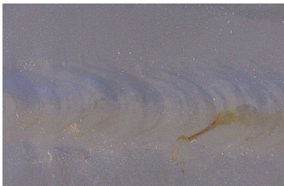
8B: Weld bead protected by synthetic paint
