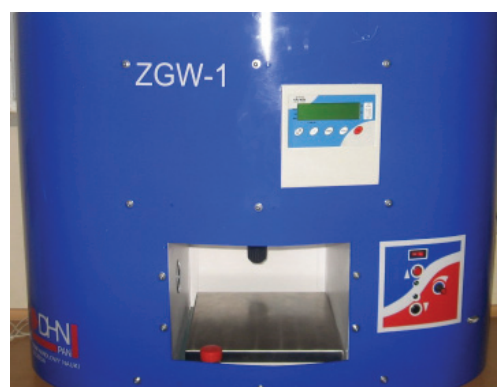
2: Hardness tester ZGW-1 used for tests
