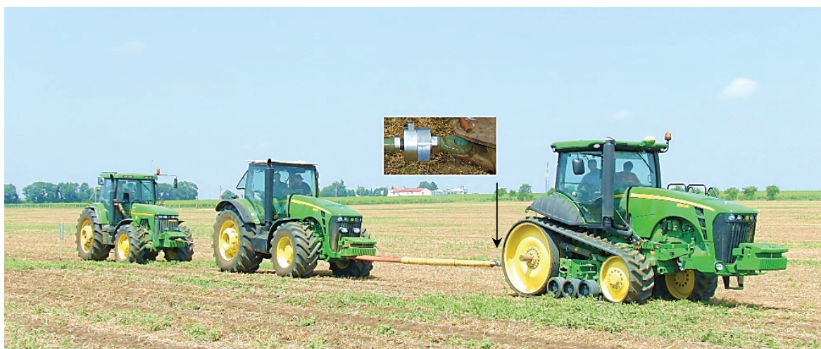
1: Set of the measured and the loading tractor interconnected by the rope containing strain-gauge sensor
