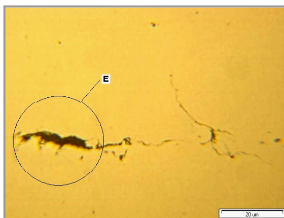
b – iniciace a rozvoj trhliny b – initiation and expansion of the crack
