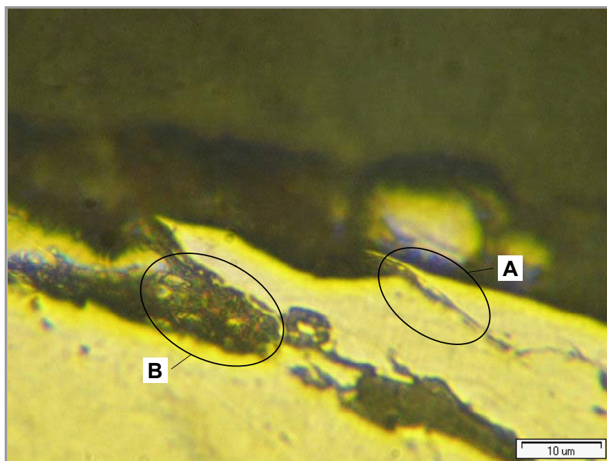
9: Rozvoj trhlin na povrchu boku zubu s různou intenzitou průniku maziva (A – nevýrazný, B – rozsáhlý) 9: Expansion of the cracks on the side surface of the teeth with the different intensity of lubricant penetration (A – lackluster, B – extensive)
